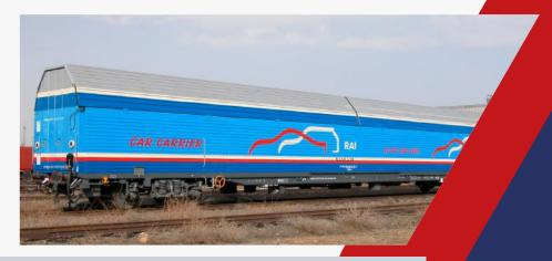
These wagons are designed for transportation of cars with the capacity of 10 cars at least or 15 tonnes load arranged according to UIC 567-4. Wagons are fully covered double deck and can be loaded from both end of the car body. Max. speed of this wagon is 160 km/h and is suitable for servicing in passenger trains.
