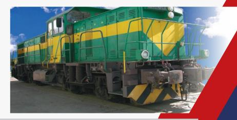
Me 10 locomotive is a multi-purpose diesel electric locomotive AC/AC for shunting and line service with the 100 km/h speed. Satisfactory operation is insured in conditions of  $-15^{\circ}$ C to  $+45^{\circ}$ C at 1800 m above sea level. Locating the driver's cab near the center ensure optimum viewing on all sides. The diagonally arranged driver's desk incorporating the power power and brake controls permits smooth operationin both directions of travel.
