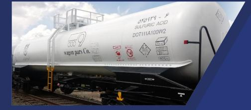
General design of the wagon is based on the standard of tank wagons according to UIC573 and this wagon is designed to carry sulfuric acid. The wagon is suitable for high speeds with a speed of 120 km/h without load and 100 km/h with load and is also equipped with a brake type and is used in SS/S type traffic.
