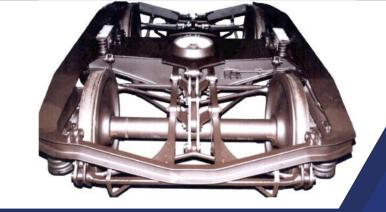
The bogie designed for international gauge and consists of a welded frame and coil spring suspension. Suspension damping is by means of a LENOIR type friction device. The axles is according to UIC 811-1 normalized and the wheel is monoblock type according to UIC 812-3. Wagon Pars Company has produced 1948 sets of bogie type Y25 for Syrian Railway and 1098 sets for RAI up to now.
