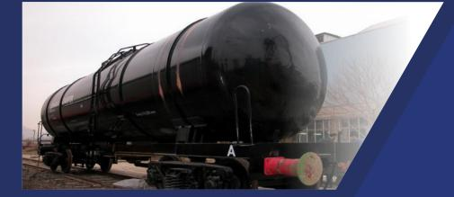
The four axlesd tank wagon is intended for transportation of light petroleum products. These products are dangerous materials and are subject to RID regulations for class 3. The wagon design guarantees enough stability during train movement. The underframe is a welded construction made of steel plates and rolled steelsections.
