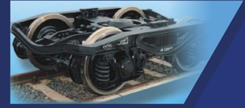
This bogie is designed on the base of ERRI-UIC standards, for freight wagons with the axles load of 22.5 tons and speed of 100 km/h that can be operated with speed of 120 km/h with axles load of 20 tons. This kind of bogie with the frame of welded structure of steel plates and profiles and casting steel has been produced by Wagon Pars Company in 2007.
